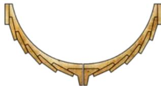
**Clinker Built Ship:** Naroo ships are called clinkers because of the style of boat building. The technique uses layers of wood, one overlapping the next to create a water tight ship.
